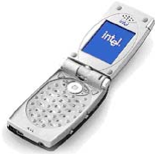
Figure 2. Prototype of an Intel XScale/Linux-based cell phone with personal server integrated (From: [3])
